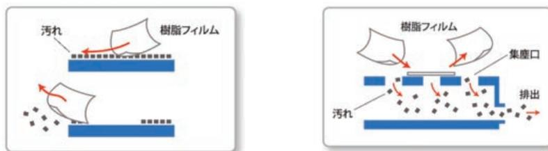
Fig. 1 Cleaning process of residual substances using plastic films.
