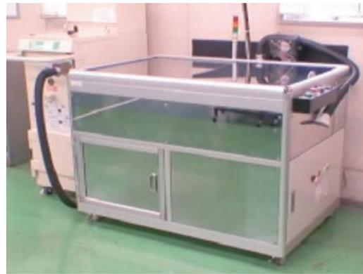
Fig. 4 Exterior view of pallet cleaner.
